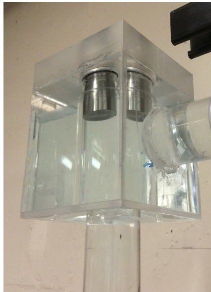
Figure 3.6: Flowing fluid study test section with no bubbles. It is possible to see how the flow must pass by the ultrasonic horn and how small the flow cross section is past the horn
